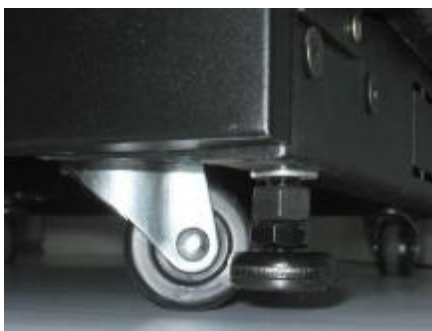
Castor Wheels and Leveling Feet
